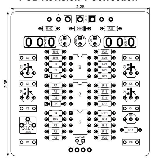
**NOTE:** Due to a silkscreen error on Revision 1 PCBs, Q1 - Q4 should be installed backwards compared to the silkscreen on the PCB when using 2N5952 transistors. (Correct pinout is marked in the image above)
