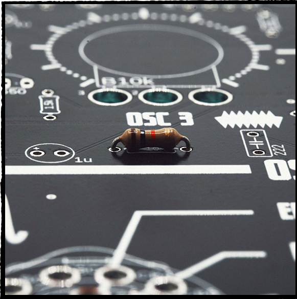
Image of resistor placed correctly.
